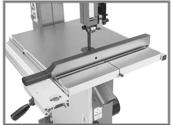
Figure 24. Example of aligning the fence with the table miter slot.
